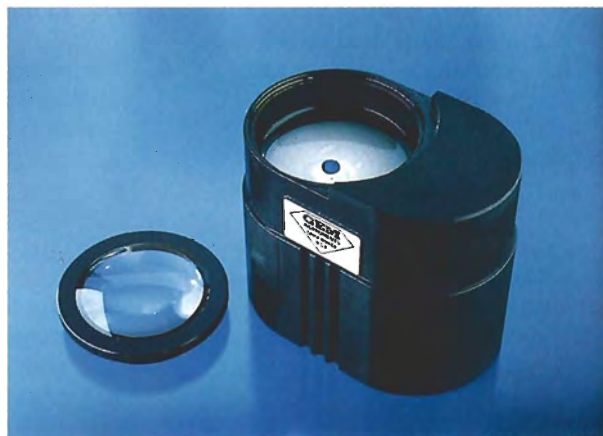
Figure 19. GIA GEM Instruments' new portable Illuminated Immersion Cell is designed to detect diffusion treatment. Photo by Maha Smith.
