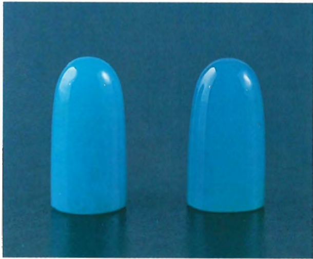
Figure 5. The 9.456-ct chrysocolla cabochon on the left is untreated; the 9.319-ct one on the right was soaked in water for several hours, with an apparent improvement in color and diaphaneity. Courtesy of Chris Boyd, CB Gems, Scottsdale, Arizona; photo by Maha Smith.
