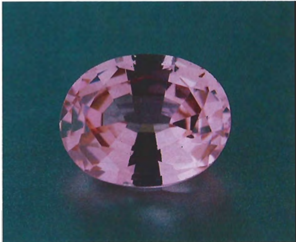
Figure 16. Titanium is the coloring agent of this 2.40-ct Czochralski-pulled synthetic pink sapphire. Photo by Maha Smith.
