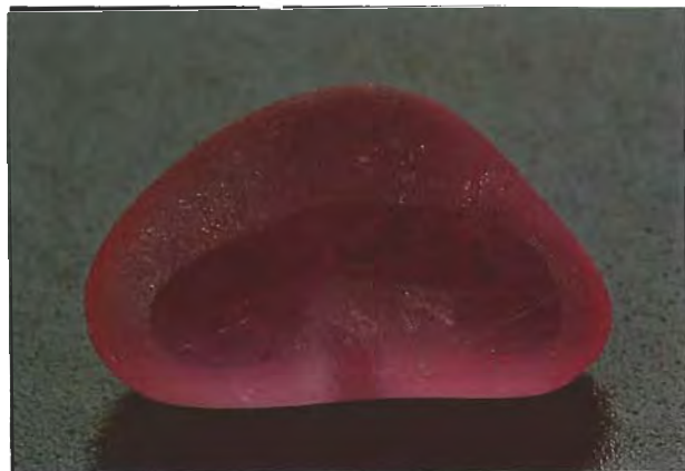
Figure 14. This convincing 6.41-ct imitation of a waterworn ruby crystal (here with optical flats cut to facilitate testing) was identified as neodymium-doped lead glass. Photo by Maha DeMaggio.
