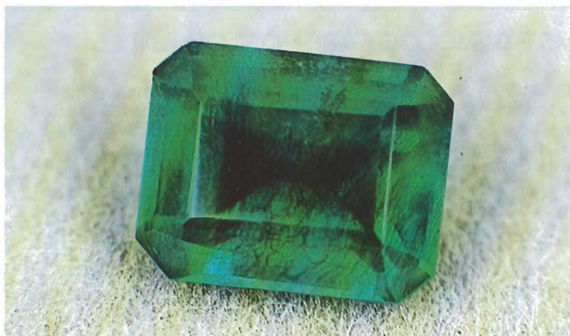
Figure 15. Dyed "crackled" green quartz, 0.96 ct.
