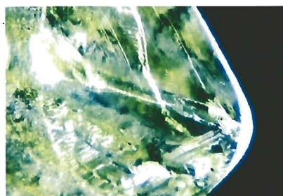
Figure 5. Green skin on a naturally irradiated rough diamond crystal. Magnified 15×.
