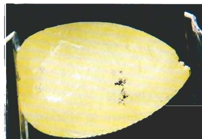
Figure 3. Badly burned diamond. Magnified 18 \times .
