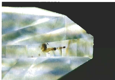
Figure 4. Brown spots on the faceted girdle of a diamond. Magnified 20×.
