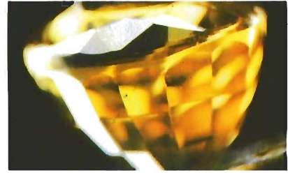
Figure 18. Multiplane girdle, thought to be typical of treated sapphire. Magnified 12×.
