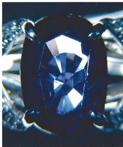
Figure 18. The abraded facet junctions on this approximately 3-ct diffusion-treated sapphire probably could not be repolished without removing part of the shallow color layer.
