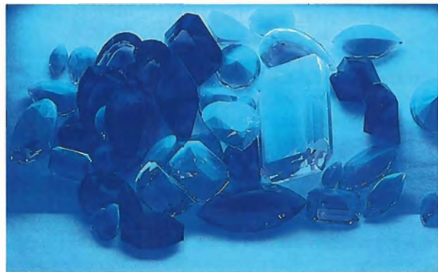
Figure 12. In this parcel, the glass imitations fluoresce chalky blue—while the amethysts are inert—to short-wave U.V. radiation.
