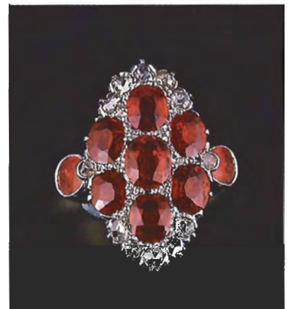
Figure 16. This beautiful period ring contains nine "Geneva rubies" (early flame-fusion synthetics). The center stone is over 1 ct; none of the stones shows strain cracks.
