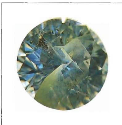
Figure 1. The filling in this 3.02-ct diamond was damaged by the heat from a jeweler's torch.
