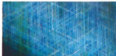
Figure 12. Rutile needles in the star quartz cabochon shown in figure 12. Magnified 30 \times .
