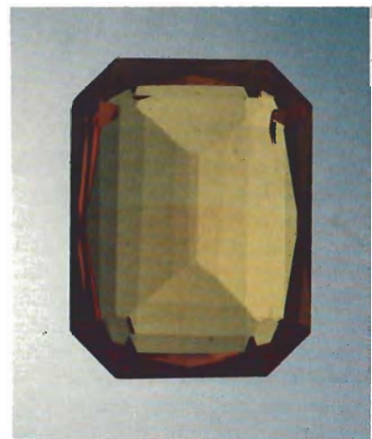
Figure 13. The curved striae in this 15.54-ct yellow flame-fusion synthetic sapphire are unusually apparent.
