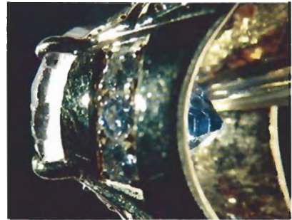
Figure 12. The concentration of color in the culet area of the synthetic sapphire shown in figure 11 lends the color to the entire stone when seen face up. Note also the unusual depth-to-width ratio of this stone.
