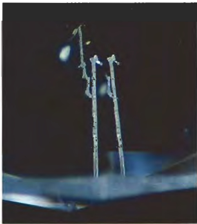
Figure 5. This laser drill hole (seen doubled due to prism reflection) goes straight from the surface to one included crystal, but also branches to a second, deeper inclusion. Magnified 63 \times .
