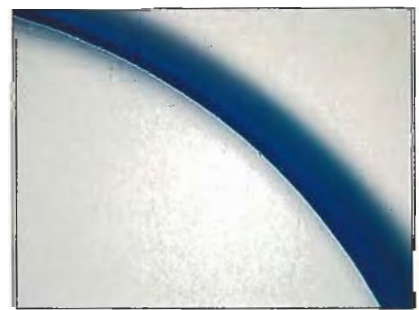
Figure 15. A slice cut from one of the beads in figure 13 confirms the thin (0.07–0.10 mm) color layer on a colorless substrate. Magnified 40 \times .
