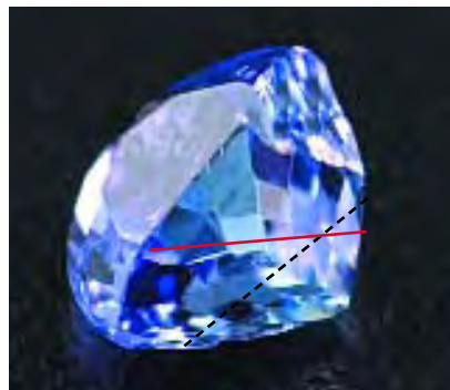
Figure 16. To investigate possible diffusion treatment, a 4.19 ct tanzanite was sawn through the center. The area close to the culet (marked by the dashed line) was lighter in color than the rest of the stone. The solid red line indicates the location of electron microprobe analyses.
