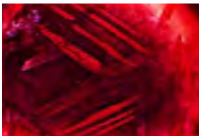
Figure 15. Precise orientation along octahedral planes suggests that these color-causing sheets of hematite might be the result of exsolution in their Sri Lankan spinel host. Magnified 10×.
