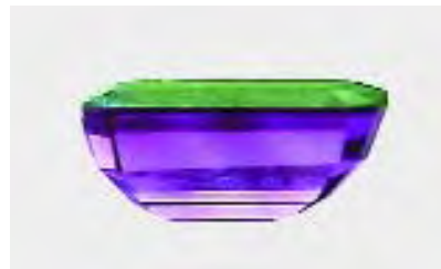
Figure 13. In profile, with diffused transmitted light, both parts of the doublet become evident, as do the curved color bands in the synthetic color-change sapphire pavilion.
