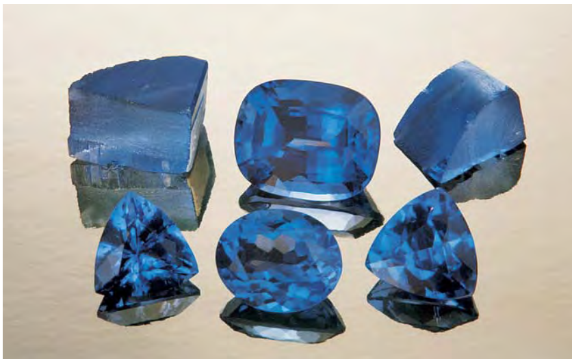
Figure 11. The strong pleochroism of this cobalt-doped synthetic forsterite makes it a convincing tanzanite imitation. The largest cushion mixed cut weighs 6.15 ct and measures 12.29 \times 9.85 \times 7.06 mm. Courtesy of Tom Chatham.
