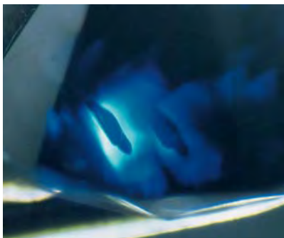
Figure 9. Magnification and fiber-optic lighting revealed both a dark blue color and a rod-shaped inclusion (typical of a metallic flux) in the synthetic diamond. Magnified 40×.
