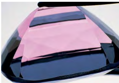
Figure 12. The two pleochroic colors displayed by the synthetic forsterite, as seen here with polarized light, were blue and purplish pink. Magnified 10 \times .
