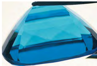
Figure 12. The two pleochroic colors displayed by the synthetic forsterite, as seen here with polarized light, were blue and purplish pink. Magnified 10 \times .
