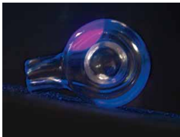
Figure 24. The zone containing the whitish bands exhibited strong pinkish purple fluorescence to short-wave UV radiation (upper left in this photo), and the edge of this zone fluoresced blue. Photo by G. Choudhary.
