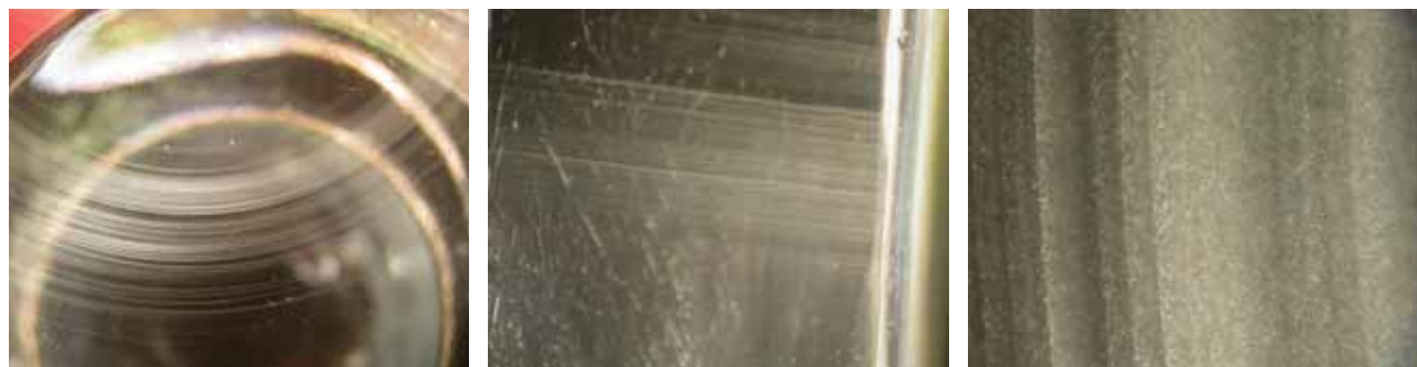
Figure 23. A zone of concentric whitish bands, similar to those seen in flame-fusion synthetic sapphire, was visible through the base of the glass object (left); note the white crystallites along the inner edge of the zone. When the glass object was viewed from the side (center), the curved whitish bands appeared as straight parallel planes, as would be expected for a cross-section through concentric cylindrical tubes. At higher magnification (right), the circular bands were seen to be composed of planes of white pinpoint inclusions. Photomicrographs by G. Choudhary; magnified 10× (left and center) and 65× (right).
