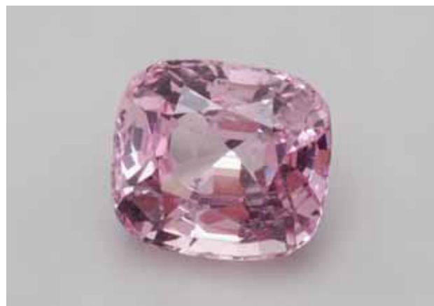
Figure 32. This unusual 15 ct flame-fusion synthetic spinel proved to be colored by iron. Photo by M. S. Krzemnicki, © SSEF.
