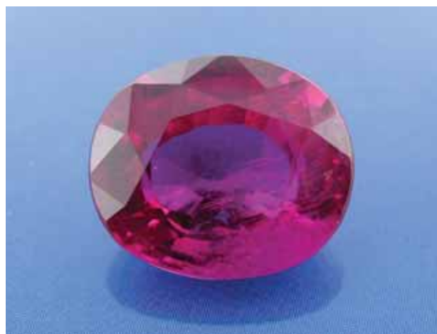
Figure 25. This 10.12 ct sample proved to be a heat-treated Kashan flux-grown synthetic ruby. Photo by S. Singhamroong, © Dubai Gemstone Laboratory.
