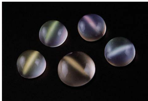
Figure 22. These five cabochons demonstrate the range of colors available in "Celestial moonstone," that is, moonstone backed with a dichroic film. They range from 5.90–6.10 × 3.85 mm to 7.90–8.00 × 4.05 mm; their total weight is 5.91 ct. Photo by Maha Tannous.
