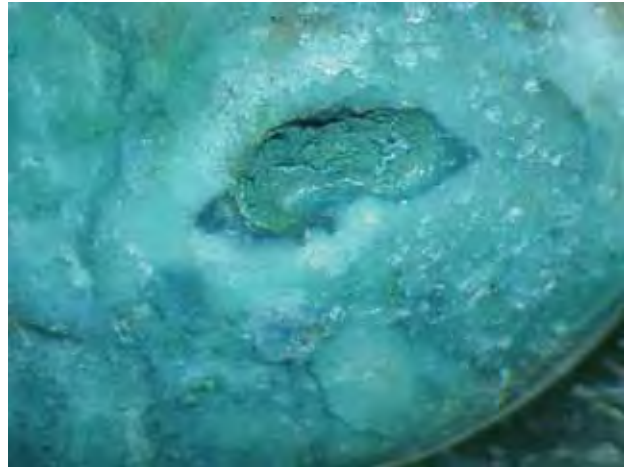
Figure 28. Microscopic examination of the dyed chalcedony shows a greenish blue dye concentrated in fractures and cavities. Photomicrograph by N. Ahmed, © Dubai Gemstone Laboratory; magnified 20 \times .
