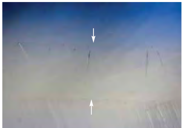
Figure 26. At higher magnification, the spicules in the seed plate appeared to be oriented in different directions. The central colorless seed plate is separated from the synthetic quartz overgrowth by sharp planes on either side (see arrows). Photomicrograph by G. Choudhary; magnified 65 \times .
