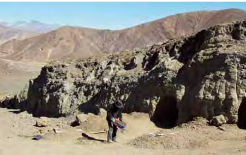
Figure 1. The andesine-bearing deposits in Tibet are exploited in a series of tunnels, with the miners using simple hand tools. Photo by A. Abduriyim.
