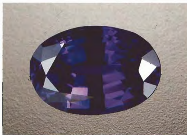
Figure 22. This 7.07 ct tanzanite imitation—which contains yttrium, aluminum, and europium—has a very convincing color. Courtesy of Bill Vance; photo by Maha DeMaggio.
