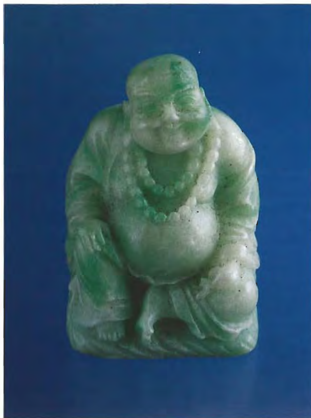
Figure 20. This 239.37 ct imitation jadeite statue ( 47.35 \times 32.90 \times 32.75 mm) is composed of finely ground calcite in a groundmass of alkyd resin polymer (plastic). The green areas were probably produced by selective dyeing. Photo by Maha DeMaggio.
