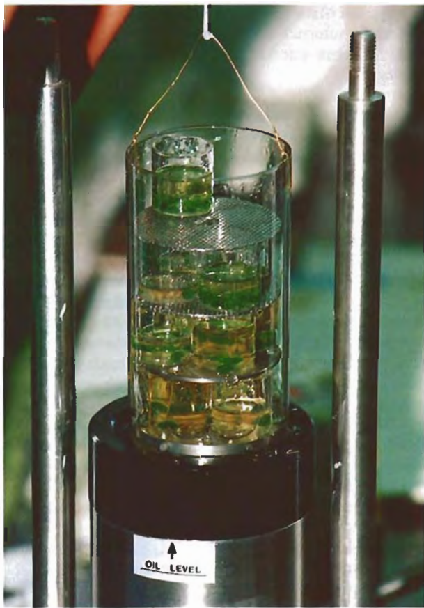
Figure 21. This unit, the larger of two “LubriGem” systems, was developed in Israel to fill fractures in emeralds.
