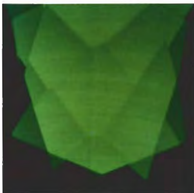
Figure 16. The use of a translucent, medium dark blue plastic filter over transmitted illumination accentuates the curved color banding in this 5.16-ct yellowish orange synthetic sapphire. Magnified 10 \times .
