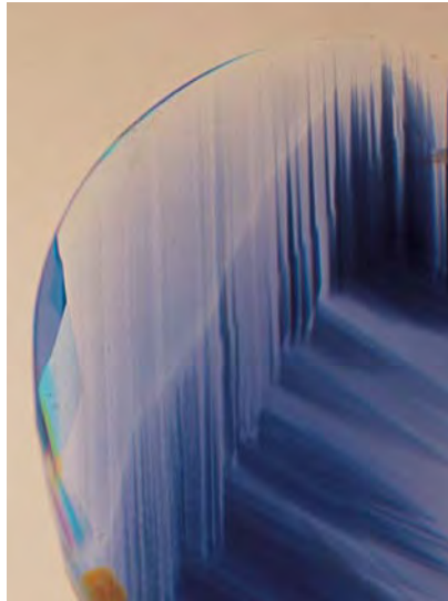
Figure 15. In many of these treated sapphires, when observed from certain orientations, the interface between the light and dark areas was marked by a colorless line all along the dark core. Immersion, magnified 12 \times .
