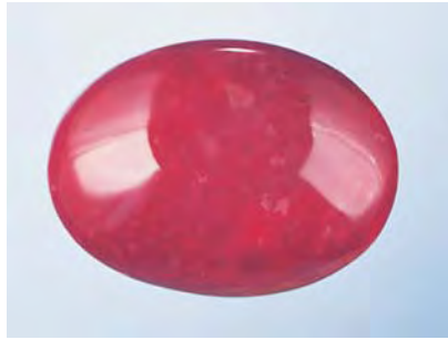
Figure 7. Represented as “pupurine,” this 43.73 ct cabochon was identified as a devitrified manufactured glass.
