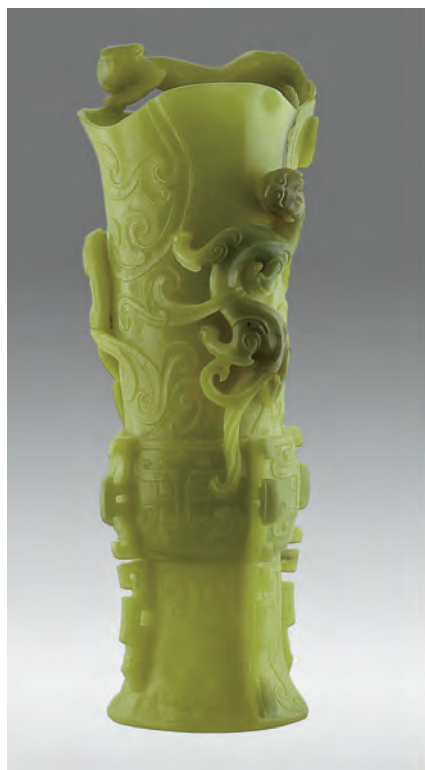
Figure 22. This 583.20 g carved vessel, composed of strontium-calcium aluminate doped with rare-earth elements, displayed a strong green phosphorescence reaction, as shown on the right.
