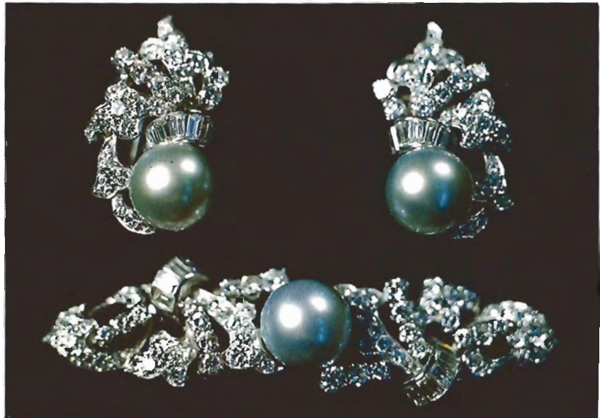
Figure 14. All three of the 12-mm gray cultured pearls in this pair of earrings and matching brooch were found to have hollow centers filled with some foreign material.
