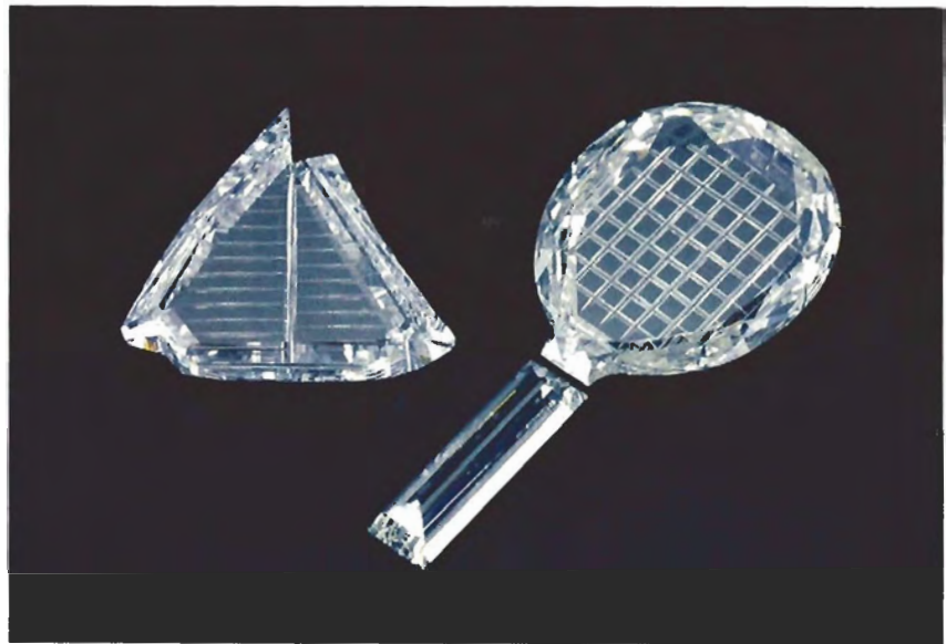
Figure 3. With the technology provided by laser sawing, fanciful cuts such as this 12-mm sailboat and tennis racket can be obtained from otherwise difficult to cut pieces of rough.
