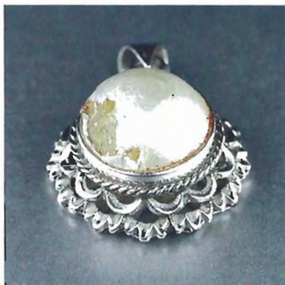
Figure 8. A damaged Mabe pearl (approximately 14 mm) with a very thin nacre shell over a wax-type filler.
