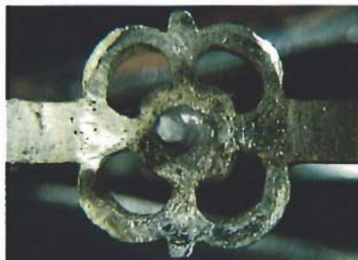
Figure 15. This metal banding undoubtedly acted like a stencil to produce the erosion pattern seen on the pearl in figure 14. Magnified 10 \times .
