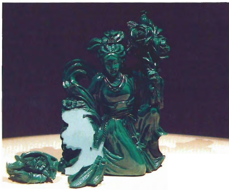
Figure 17. Damaged malachite carving showing separation between bedding planes; 2.5 cm \times 7.5 cm \times 10.5 cm high.
