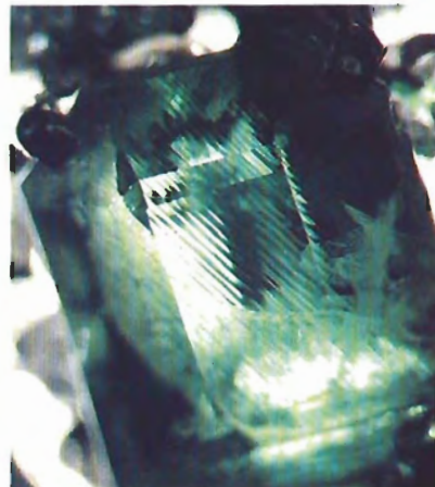
Figure 16. "Venetian blind" banding in synthetic emerald. Magnified 10 \times .
