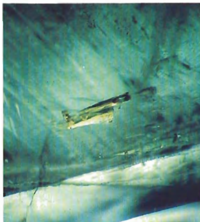
Figure 15. Yellow inclusion in a synthetic emerald. Magnified 25 \times .
