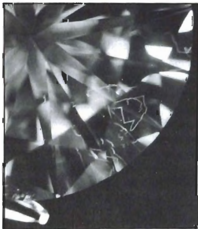
Figure 8. Irregular tube-like inclusions in a diamond. Magnified 18 \times .
