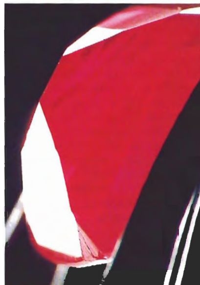
Figure 20. Angular banding in a flux-grown synthetic ruby. Magnified 30 \times .
