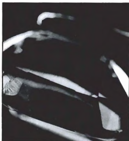
Figure 21. Curved striae and "fingerprint" inclusions in synthetic ruby. Magnified 30 \times .
