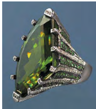
Figure 8. The large dark yellowish green modified shield cut in this ring exhibits high dispersion. Although it was purchased as a peridot, advanced testing identified it as glass.
