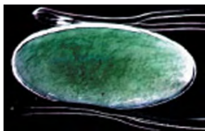
Figure 10. In transmitted light, the dye concentrations in this 5.65 ct jadeite cabochon could be seen surrounding individual grains, as well as filling surface-reaching cracks and fractures.
