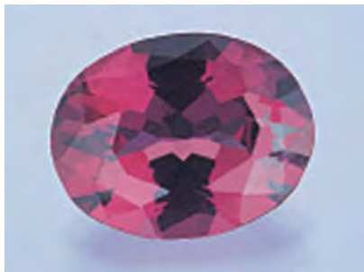
Figure 17. This 8.38 ct purple-pink spinel proved to be of natural origin based on its photoluminescence spectra.
