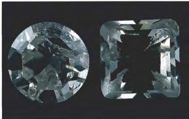
Figure 5. These two diamonds, a 16.48 ct blocked round and an 18.15 ct blocked square, were cut from the same piece of rough, both fractured due to strain.
