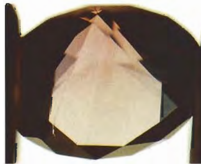
Figure 10. The streaky pink color seen in this 0.05 ct treated-color pink diamond might be confused with the pink graining seen in natural-color diamonds. Examination at 10× to while the stone was immersed in methylene iodide reveals that the color is largely confined to the surface.
