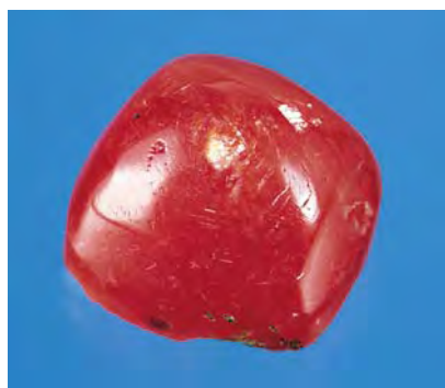
Figure 1. This 10.45 ct orange-red calcite is colored by inclusions of chalcotrichite, a fibrous variety of cuprite.
