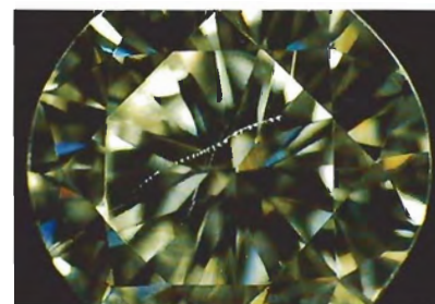
Figure 7. Even diamonds can be damaged by scratch hardness tests, as this 0.80-ct stone proves; its clarity went from VVS 1 to VS 2 . Magnified 20 \times .
