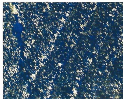
Figure 10. Banding is also evident in this thin section of the lapis cabochon shown in figure 8. Magnified 80x.
