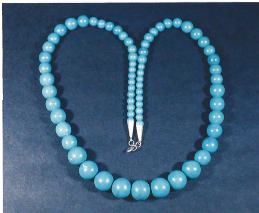
Figure 18. This imitation turquoise necklace is actually gibbsite; the beads range from 5.7 to 14.5 mm in diameter.
