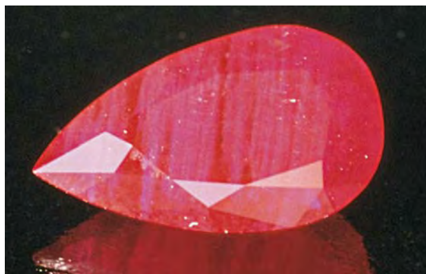
Figure 39. The 4.17 ct pear-shaped synthetic ruby cut from the "crystal" shown in figure 38 appears to contain zones of "silk," which give it a natural appearance to the unaided eye. Photo by Jaroslav Hyrsl.
