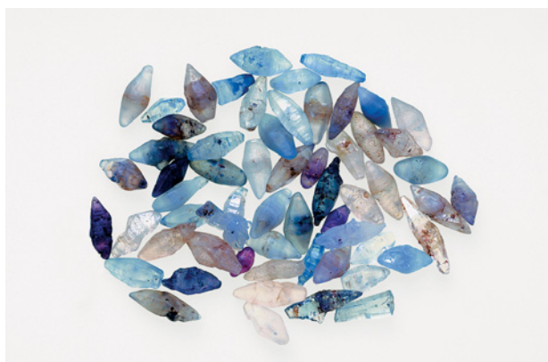
These sapphire crystals (0.08–0.40 g) from Ratnapura, Sri Lanka, were analyzed by LIBS. Courtesy of Materialytics.
