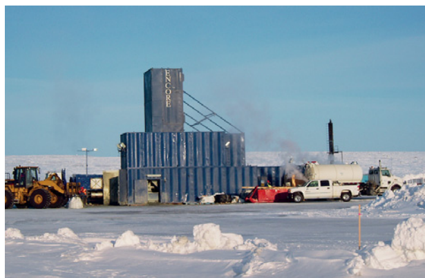
Shown here is a kimberlite bulk sampling operation (large diameter drilling) at the DO-27 kimberlite, Northwest Territories, Canada, in March 2006. Photo by H. G. Coopersmith.
