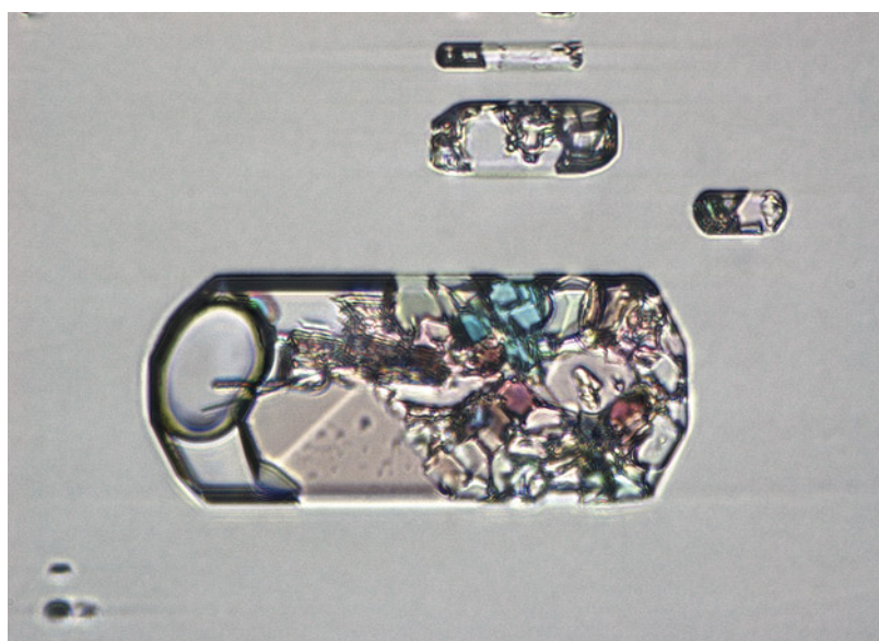
Figure 7. Fluid inclusions with exsolved gas bubbles and daughter crystals in a beryl host. These fluid inclusions entered the host through a fracture. The fracture healed itself, trapping blebs of this fluid with the negative crystal form seen here. Photomicrograph by Nathan Renfro.
