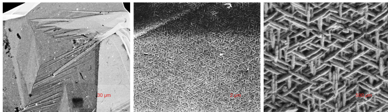
Figure 7. FESEM images of a freshly fractured iridescent hematite surface, shown with increasing magnification from left to right, reveal that the granoblastic texture of a single hematite grain (left) comprises individual nanocrystals oriented at 120^\circ angles (center and right).
