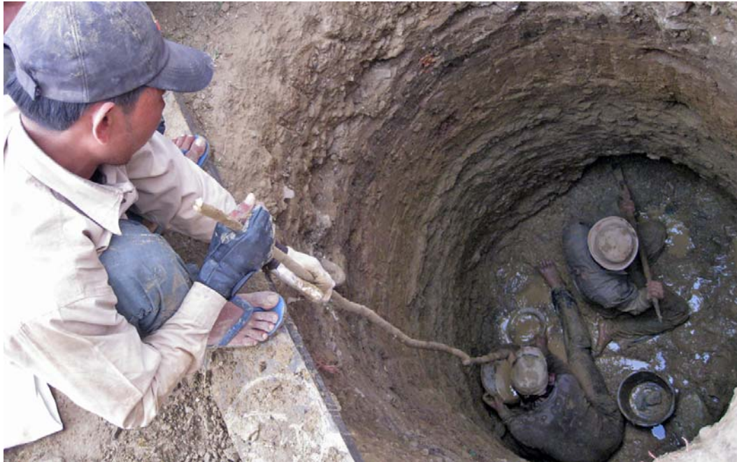
Figure 19: Recovering potentially gem rich gravels at Mr. S. mine in downtown Pailin. Photo: V. Pardieu, 2008
