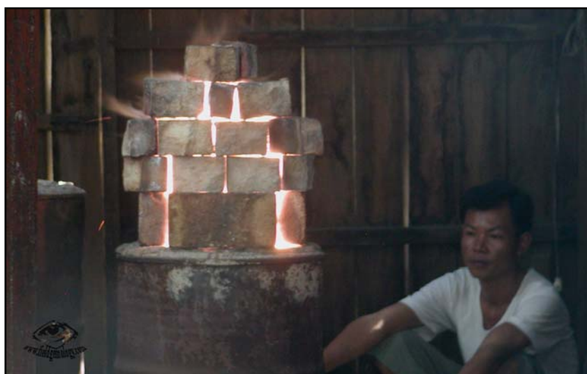
Figure 12: A Pailin burner performing heat treatment under reducing conditions on some of VP's stones, Photo: V. Pardieu, 2004
