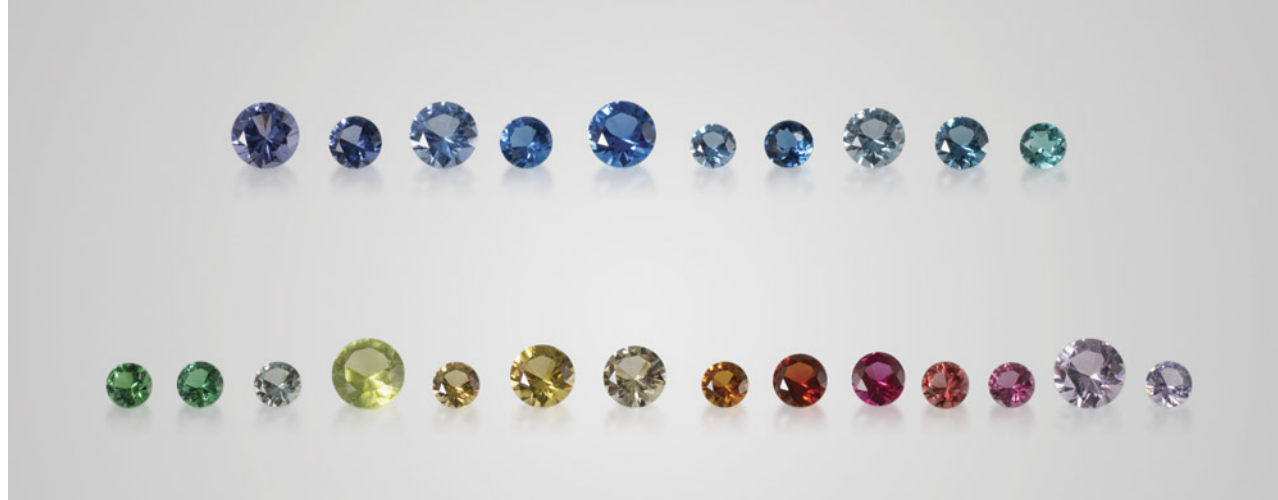
Figure 1. Glass-ceramics can be created in a full spectrum of colors to imitate a wide range of natural gemstones. Shown here are transparent samples (0.10–0.37 ct) donated for this study by the Formica Group, from left to right: GC-01 to GC-10 (top row) and GC-11 to GC-24 (bottom row). Photo by Nuttapol Kitdee.
