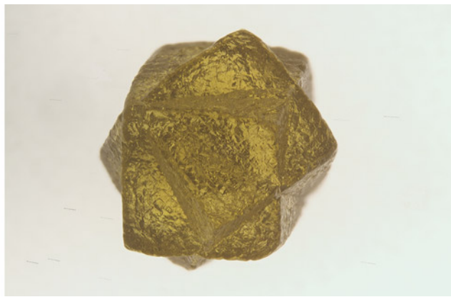
Figure 4. Left: The twinned 0.37 ct diamond displays a vivid orange yellow color. Right: The intersection of cuboid crystals is clearly observed from this view. Photomicrographs by Taryn Linzmeyer; field of view 7.19 mm.
