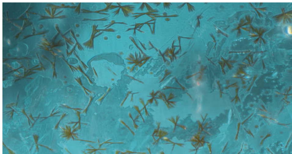
Figure 1. Goethite sprays in an apatite's surface-reaching fracture. Photomicrograph by Michaela Damba and John Koivula; field of view 1.26 mm.
