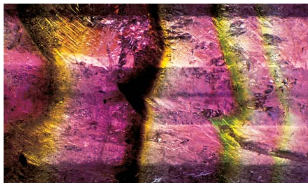
Figure 18. Oscillatory (narrow, repeating) zoning is shown by this parti-colored tourmaline that is probably from Anjanabonoina. Note the gradation in pink color intensity within each color zone, and the sharp boundaries with the green layers. Photomicrograph by John I. Koivula; magnified 10 \times .
